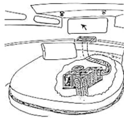
Mount unit under bed. To ensure silent running, use HFL return air aperture system with flexible ducting. Dimension return air box sufficiently large to ensure slow airspeed and good return air filtering. Air outlet box high or alternatively on 30 degree wedge at middle height.
